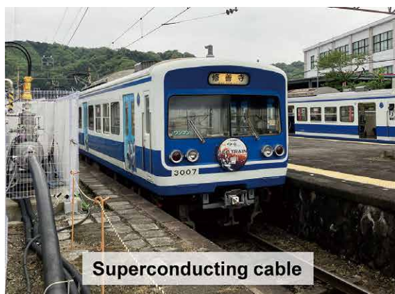
Fig. 1 Train running through a power supply section consisting of the superconducting feeding system (long-term operation on the Sunzu Line)
