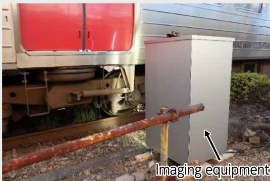
(b) Imaging equipment capturing a passing vehicle
