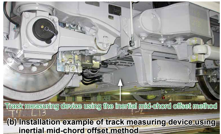
Track measuring device with the inertial mid-chord offset method
