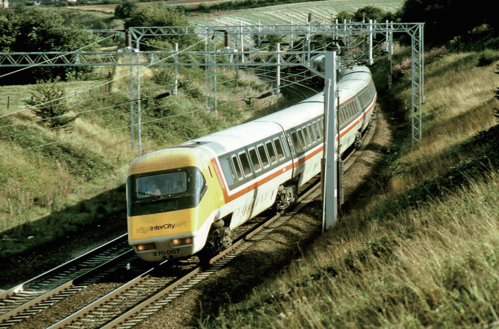
The Advance Passenger Train: an underfunded and over complex attempt to overcome the sinuous nature of old track by a sophisticated train.
