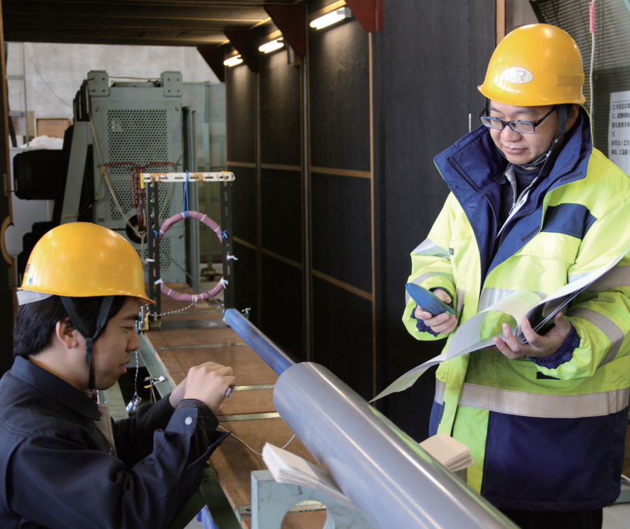
A scale model test demonstrates that the tunnel hood mitigates a spike of micro pressure wave.
