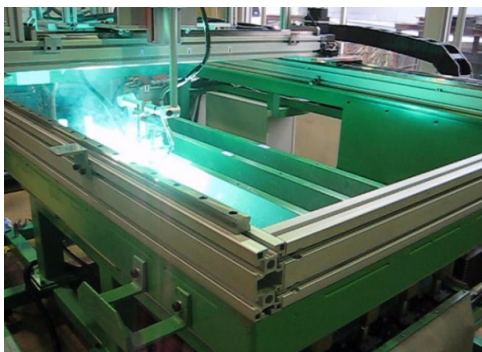
MIG welding by an automatic welding machine
