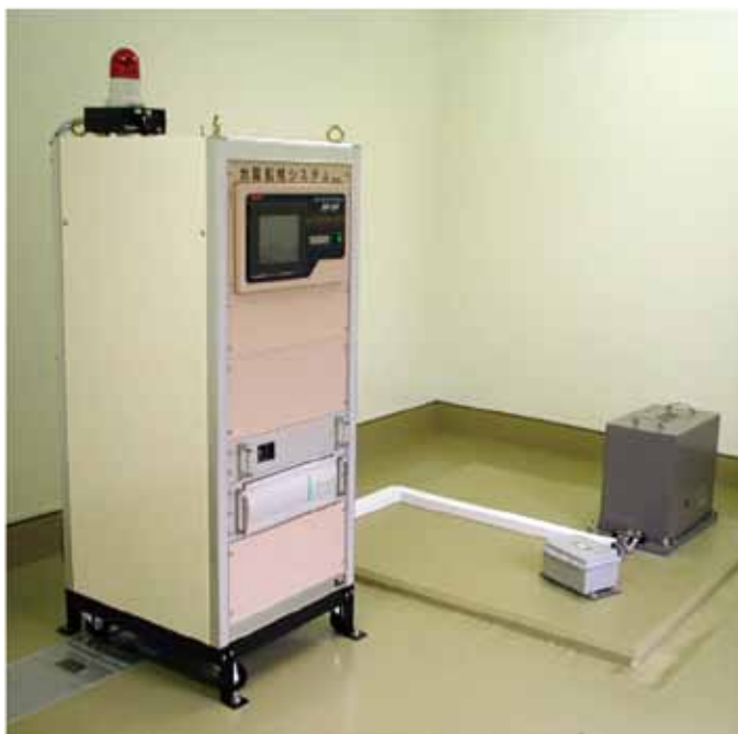
Seismometers developed for the early-warning purpose are installed at each of the detection points of the Earthquake Early Warning System. These seismometers are composed of sensors and data-processing devices which process the P-wave data detected by the sensors and issue warnings.
