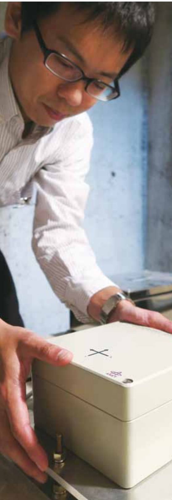
Detection points are located along railway tracks or quiet places distant from tracks. Constant temperature and humidity are maintained inside the buildings housing seismometers in order to ensure stable operation of the seismometers over a long period.
