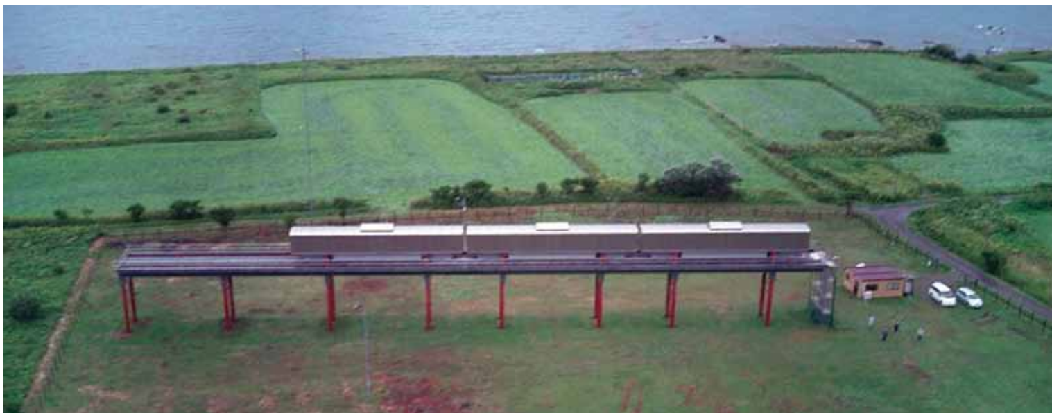
A mock-up of train consisted of three vehicles is installed on an eight-meter viaduct of single track to measure acting force due to natural wind. This site, Shimamaki village, Hokkaido, is known as an area of strong wind.
