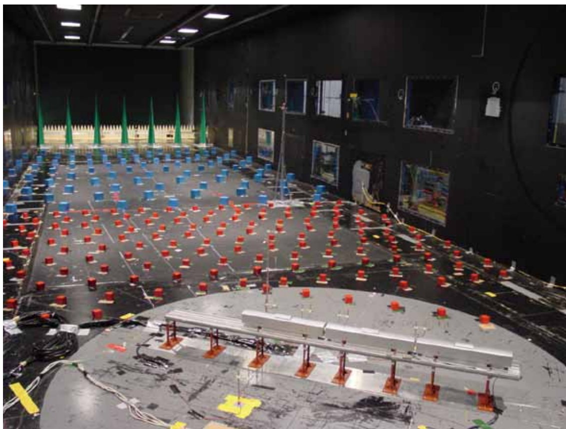
Four kinds of objects (white barriers, green spires, blue and red blocks) can generate an airflow similar to the natural turbulence. Models of a viaduct and vehicles with a scale of 1 /40 are installed on a turntable which allows to blow in different attack of angles on them. A balance set inside one of vehicle models measures forces acting on it. The wind tunnel test are in agreement on measured forces with that of the full-scale models in the field.
