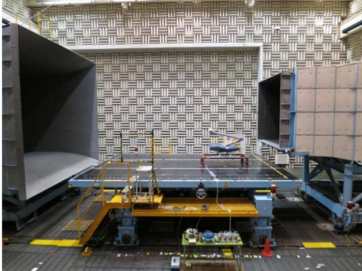
Left: Testing aerodynamic performance of an actual pantograph in RTRI's large-scale wind tunnel Right: Simulation of air flow by RTRI's supercomputer (courtesy of JR East)
