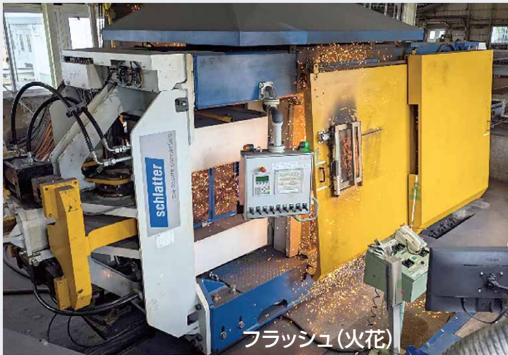
(a) 溶接状況
