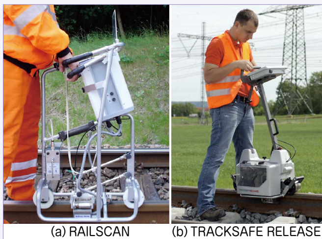
図8 RAILSCAN, TRACKSAFE RELEASEによる軸力測定 7) 提供：Electro Thermit GmbH & Co.KG, member of Goldschmidt Thermit Group
