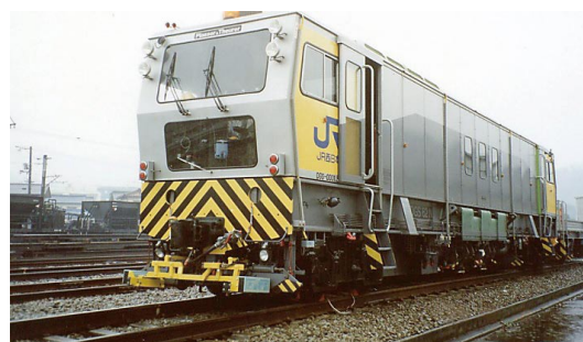
図4 DTS (Dynamic Track Stabilizer)
