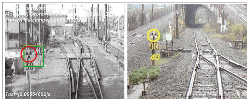
図4 徐行予告信号機の検知例
