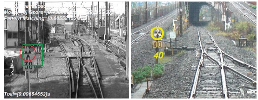
図10 徐行予告信号機の検知例
