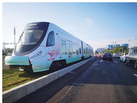
図7 仏山の燃料電池路面電車の外観 (Image provided by Ballard Power Systems)
