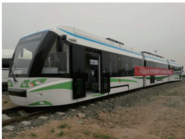
図7 唐山軌道客車の燃料電池路面電車試作車の外観 (Image provided by Ballard Power Systems)
