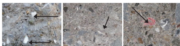
(a)エポキシ樹脂 (b) SMC成形樹脂 (c) RIM成形樹脂
