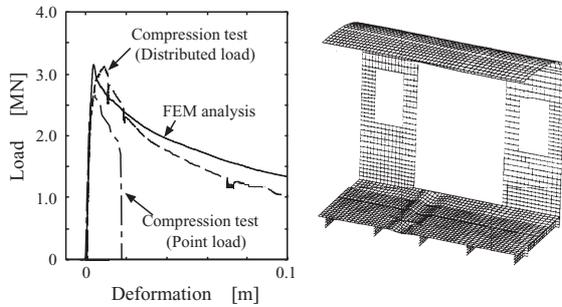
**Fig. 3 Compression load and deformation relation for the door section**
