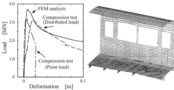
**Fig. 4 Compression load and deformation relation for the seat section**
