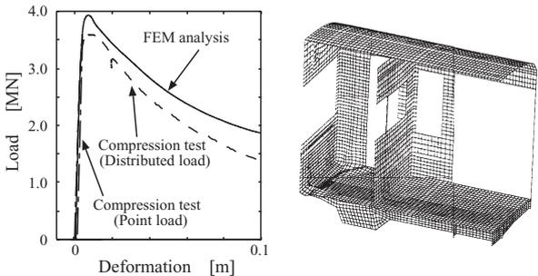
**Fig. 5 Compression load and deformation relation for the cab section**
