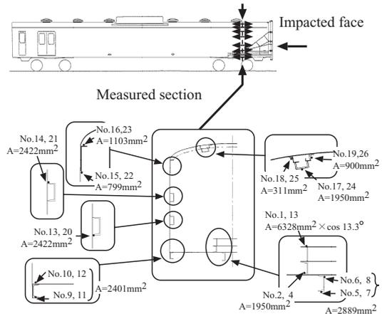
Fig. 13 Measuring points of strain in the carbody sections
