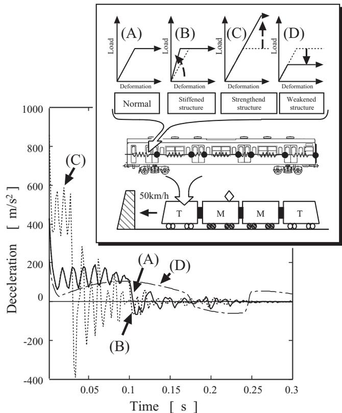
**Fig. 10 Evaluation of the impacting behaviours in changing the cab end structure**
