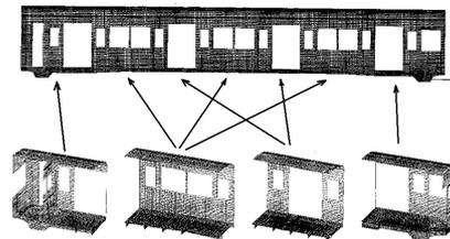
**Fig. 7 Three-dimensional FE model for a leading carriage of commuter EMU**
