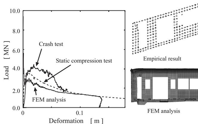
**Fig. 15 Comparison of the result from the train crash test and FE analysis**
