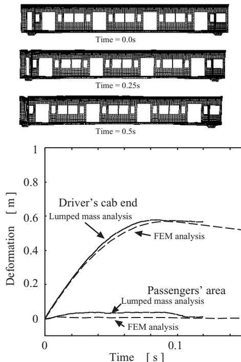
**Fig. 9 Comparison of the results of both lumped mass analysis and FE analysis**
