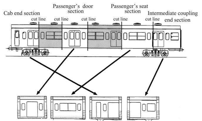
**Fig. 1 Partial carbody structures for quasi-static compression tests**
