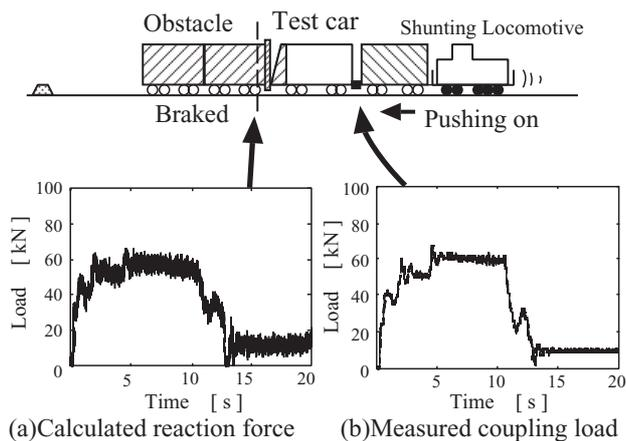
**Fig. 14 Comparison of the compression load calculated from measured values of strain of carbody structures and measured at the coupler between carriages in the impacting rake**
