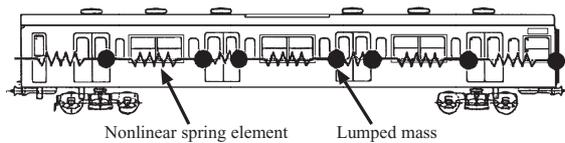
**Fig. 8 One-dimensional lumped mass modeling for a leading carriage of EMU**
