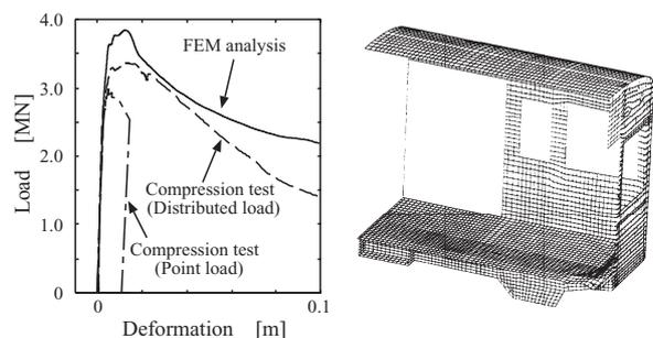
**Fig. 6 Compression load and deformation relation for the coupling end section**
