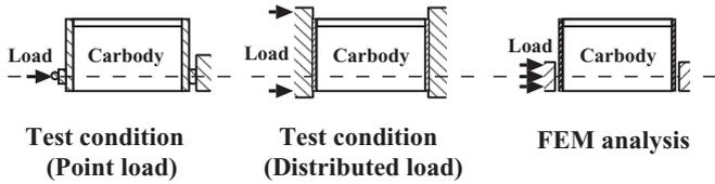
**Fig. 2 Loading condition used in quasi-static compression tests and FE analysis**
